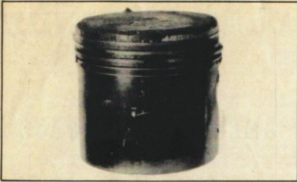
Sludge is one of the reasons oil rings clog up and prevent proper oil control with the resulting low oil mileage.
